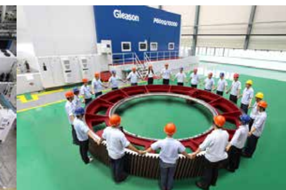
GERMANY GLEASON-PFAUTER NC-HOBBING 10-meter in China High Efficiency and Precision Hobbing Machine, Max. machining diameter 10 meters
